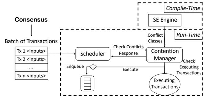
Figure 1: Architecture of System
