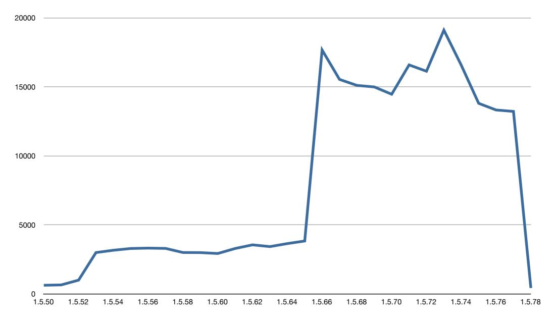
Time in ms to perform an RPC with 20Mbyte of data with each OpenAFS version
