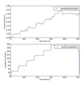
Stress test with UDP buffer size set to 16MB. In practice for the end-users working interactively the service is slightly slowed down.
