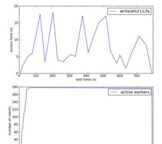
High access latency (write) reproduced in the test environment for 6 x 30 test jobs on Ixbatch. OpenAFS 1.4.14 +CERN. In practice for the end-users working interactively the service is unavailable.
