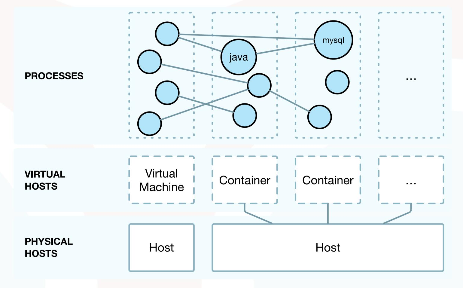
Representation of the architecture and interactions between components of a distributed system. The graph of processes illustrates the interactions of running processes.
